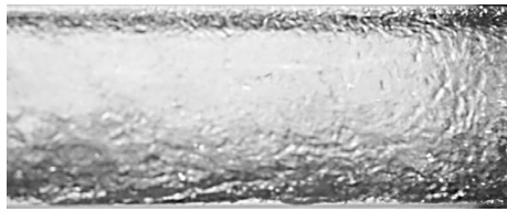
Figure 2.7: Intermittent flow - between slugs
